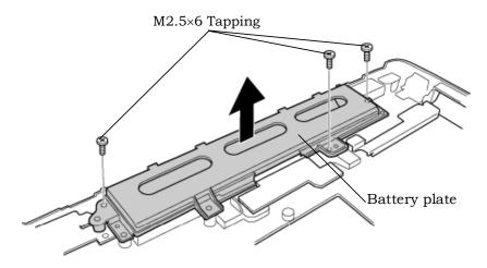
Figure 4-35 Removing the battery plate
